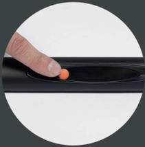
**STEP 1:** Turn the device on by lightly pressing the button. Do not move the device during calibration (about 20 sec) or it will turn itself off.
